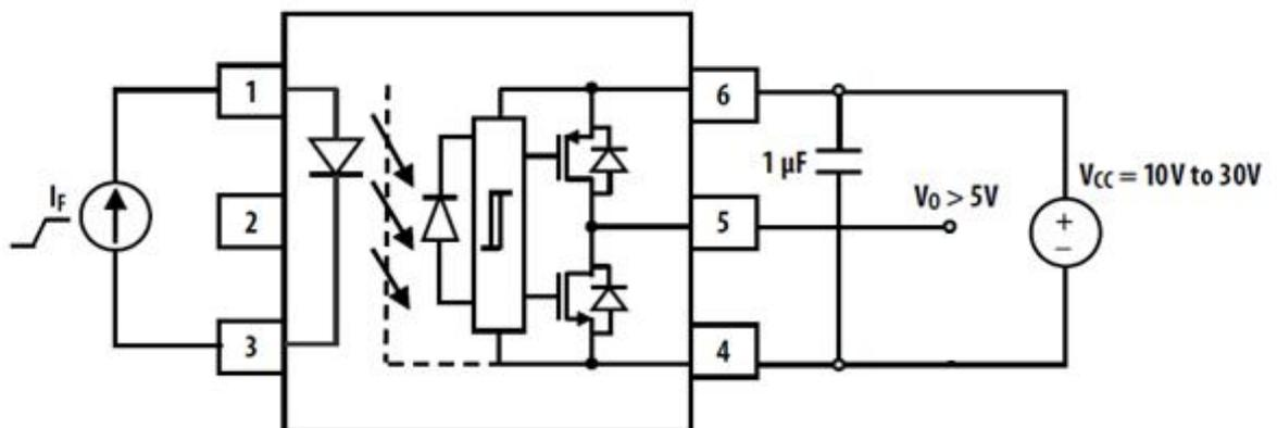
**Fig.18 I<sub>FLH</sub> Test Circuit**
