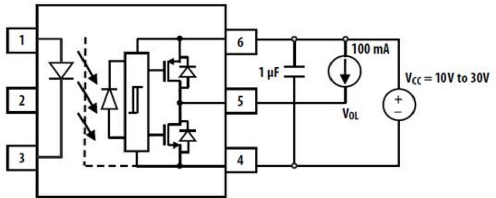
**Fig.17 V<sub>OL</sub> Test Circuit**
