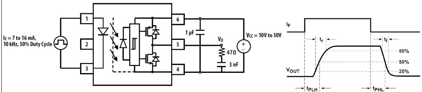
**Fig.20 tPHL, tPLH, tr and tf Test Circuit and Waveforms**
