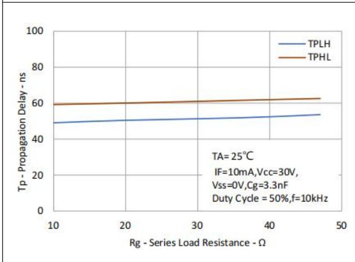
**Fig.11 Propagation Delays vs. Rg**
