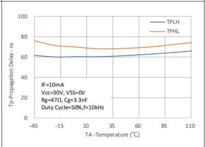
**Fig.10 Propagation Delays vs. Temperature**
