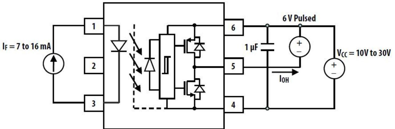
**Fig.14  $I_{OH}$  Test Circuit**
