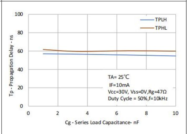
**Fig.12 Propagation Delays vs. Cg**
