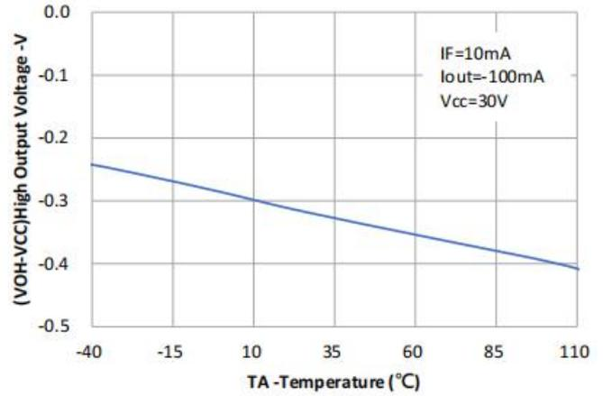
**Fig.2  $V_{OH}$  vs. Temperature**
