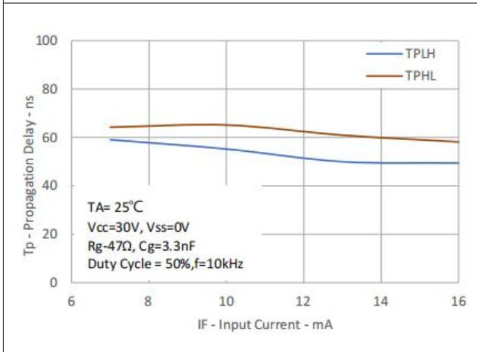
**Fig.9 Propagation Delays vs. IF**
