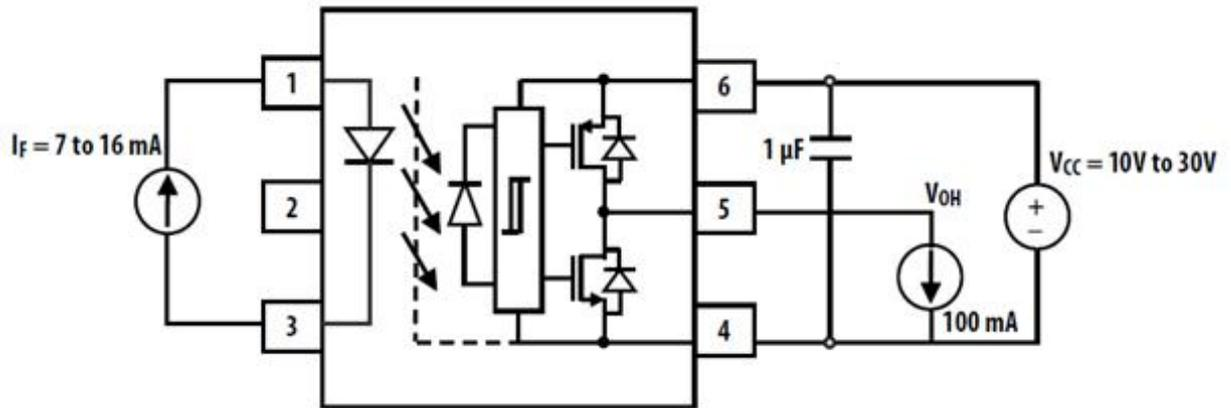
**Fig.16 V<sub>OH</sub> Test Circuit**
