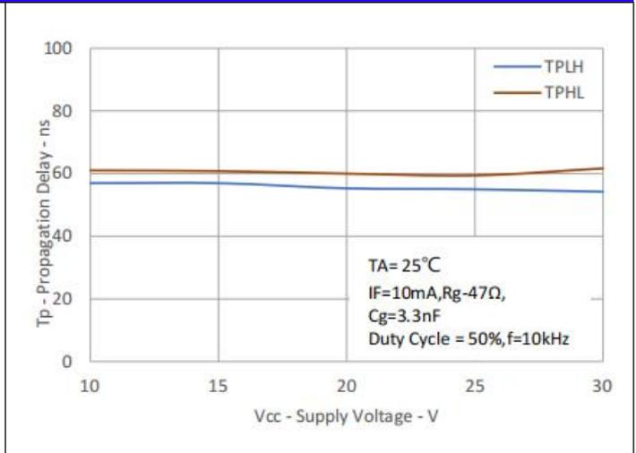
**Fig.8 Propagation Delays vs. VCC**
