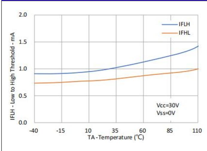
**Fig.7 IFH vs. Temperature**
